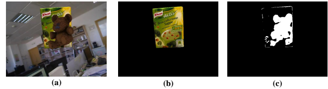
Fig. 5. Occlusion Detection. (a) A heavily occluded frame from Rigid Pose Dataset [11]. The tracked box is largely occluded by the teddy bear. (b) The template rendered with tracked pose from last frame. The rendered template is always clear and non-occluded, which contributes to a simple but efficient occlusion detection strategy. (c) The detected occlusion area. Pixels inside the area are discarded from pose tracking optimization.
